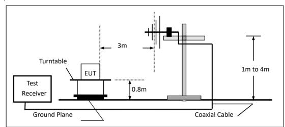
(c) For radiated emissions above 1000MHz
