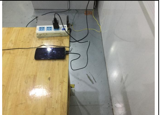
Conducted Emissions Test Setup Side View
