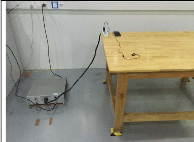
Conducted Emissions Test Setup Front View
