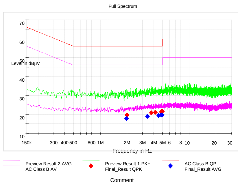
Pic1. Conducted emission L and N Line
