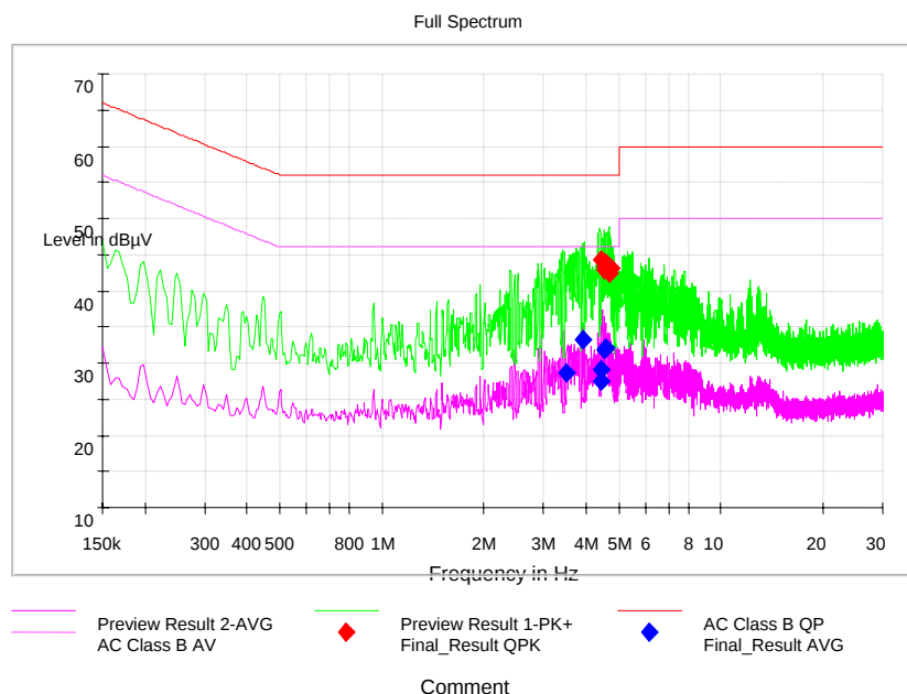
Pic3. Conducted emission N Line
