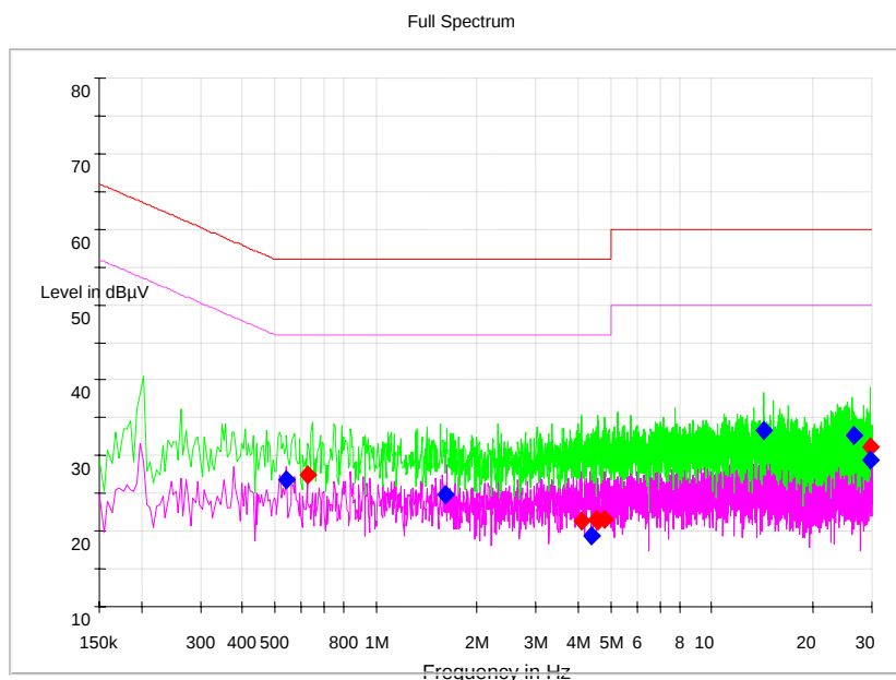
Pic5. Conducted emission N Line
