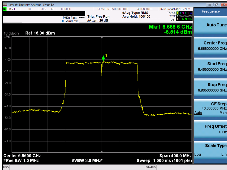
Plot 7-73. Power Spectral Density MIMO ANT1 (160MHz 802.11ax/be (UNII Band 7) – Ch. 143) - LPI
