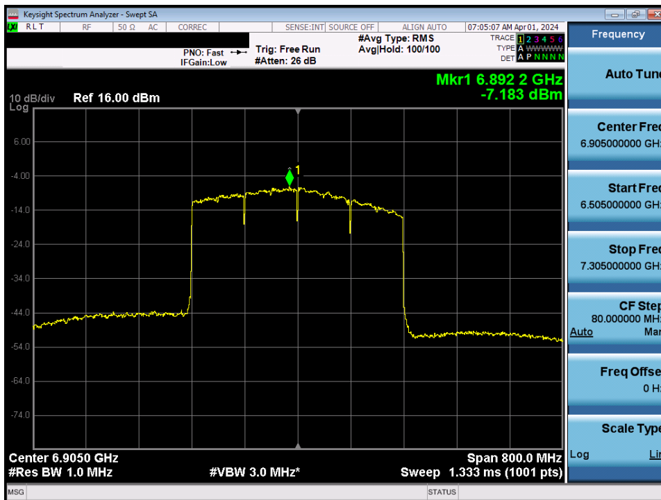
Plot 7-86. Power Spectral Density MIMO ANT1 (320MHz 802.11ax/be (UNII Band 7/8) – Ch. 191) - LPI
