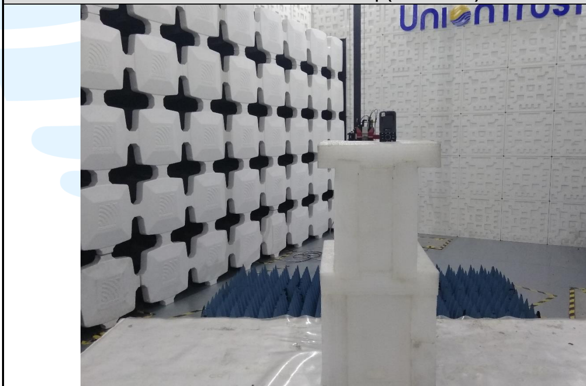
Radiated emission Test Setup (Above 1 GHz)
