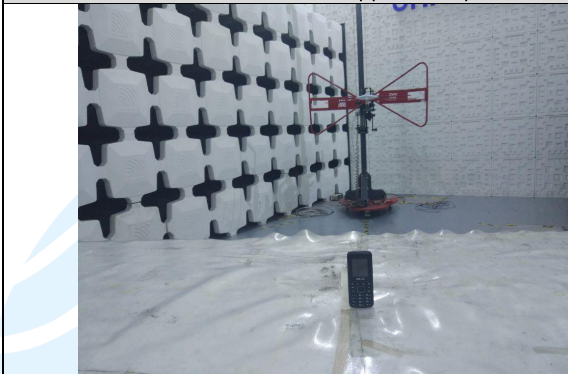
Radiated emission Test Setup (30 MHz~1 GHz)
