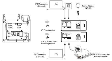
The IP phone should be used with Yealink original power adapter (5 V/0.6 A) only. The use of the third-party power adapter may cause the damage to the phone. If you are connecting a PC to your phone, we recommend that you use the Ethernet cable provided by Yealink.
