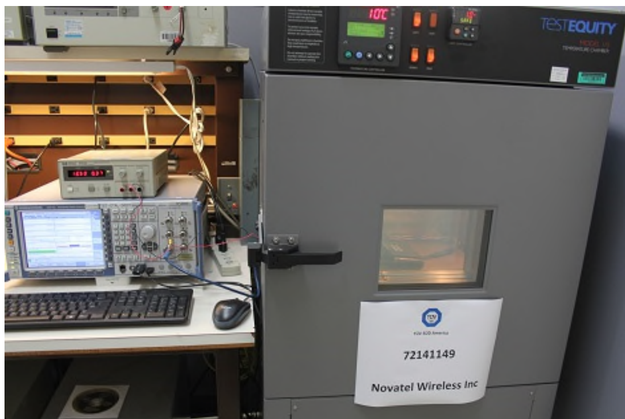
Frequency Stability Test Setup
