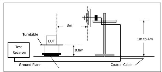
(c) For radiated emissions above 1000MHz
