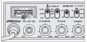
2 Full @ counterclockwise rotation opens the "gate" allowing all signals in.
