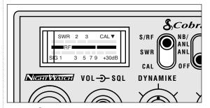
1 The S/RF-SWR-CAL switch must be in the S/RF position.
