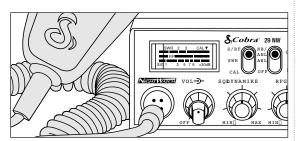
8 Attach the 4-pin microphone cable to receptacle on front of unit and Install unit in bracket securely.
