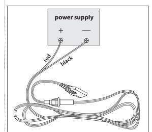
Simply connect the red (+) and black (-) leads of the transceiver to the corresponding terminals of the power supply.
