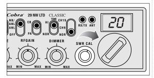
4 While holding mic button *adjust* the 🔘 SWR CAL knob so the meter needle swings to the CAL ▼ mark on the meter (located on the right).
