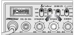
Rotate the RF Gain knob counterclockwise to reduce gain in strong signal areas. In weak signal areas turn clockwise to increase gain.
