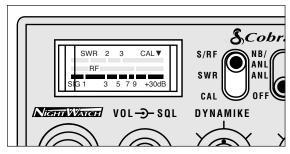
• The S/RF-SWR-CAL switch must be in the S/RF position to read the meter.
