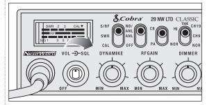
1 Rotate the On/Off Volume knob *clockwise* the green RX/TX LED will be illuminated.
