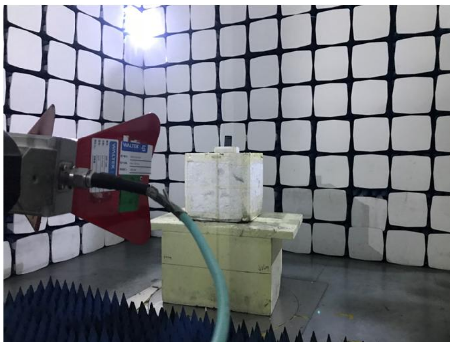
Radiation Emission Test Setup (1GHz to 18GHz)
