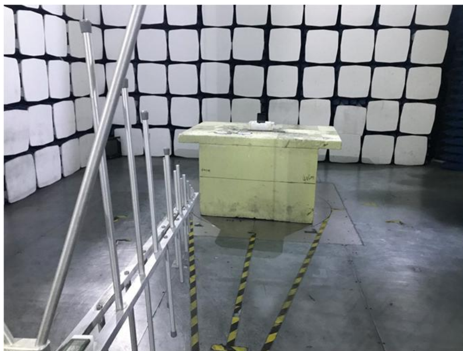
Radiation Emission Test Setup (30MHz to 1GHz)
