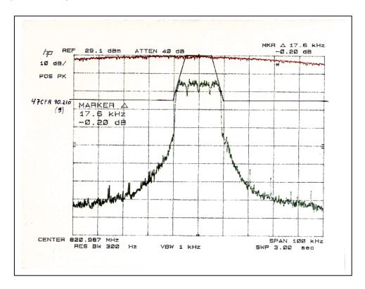
Spectrum Analyzer Plot: Emission Mask G: Tx @ 821 MHz
