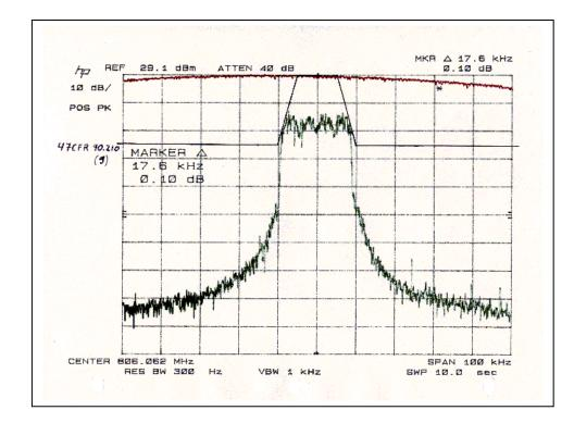
Spectrum Analyzer Plot: Emission Mask G: Tx @ 806 MHz
