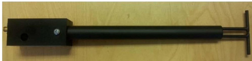
Figure 1 – MVG COMOSAR Validation Dipole
