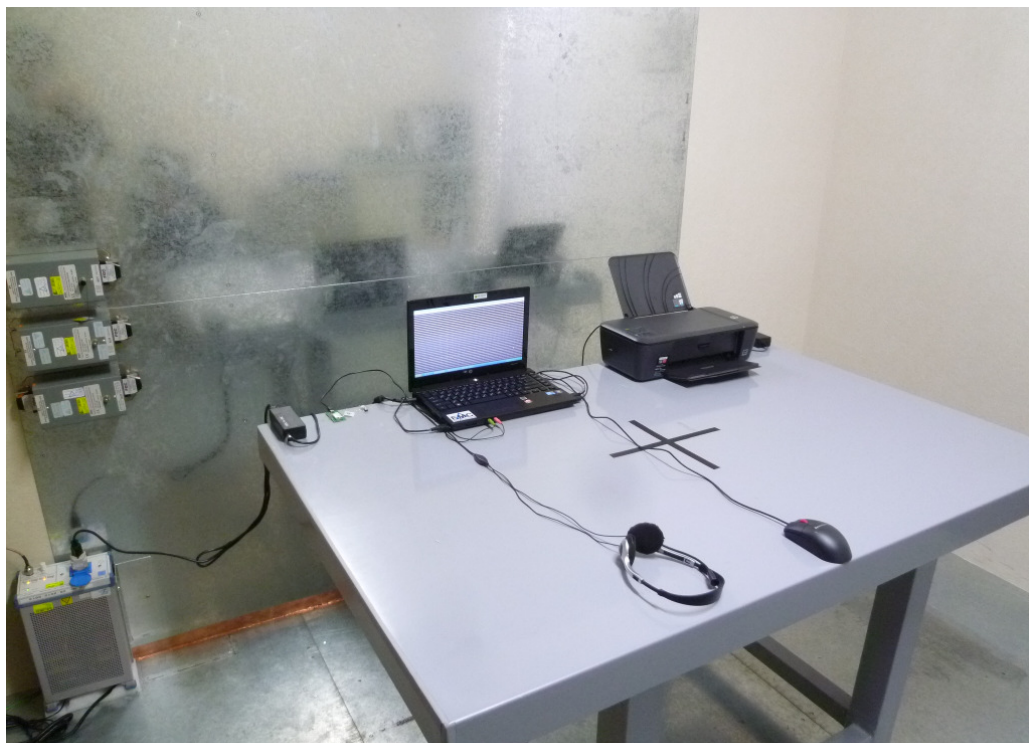
Photograph 6: Set-up for for Mains Conducted testing Front
