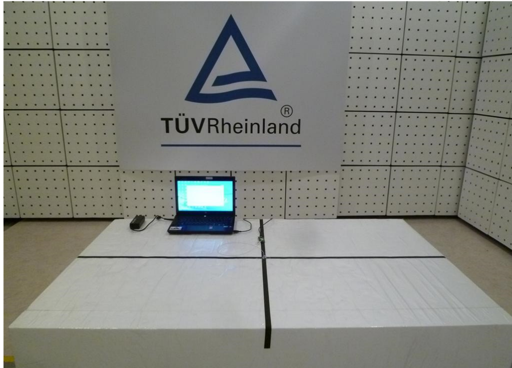
Photograph 1: Set-up for Spurious Emissions (Front View)
