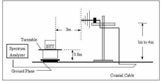
(C) Radiated Emission Test-Up Frequency Above 1GHz
