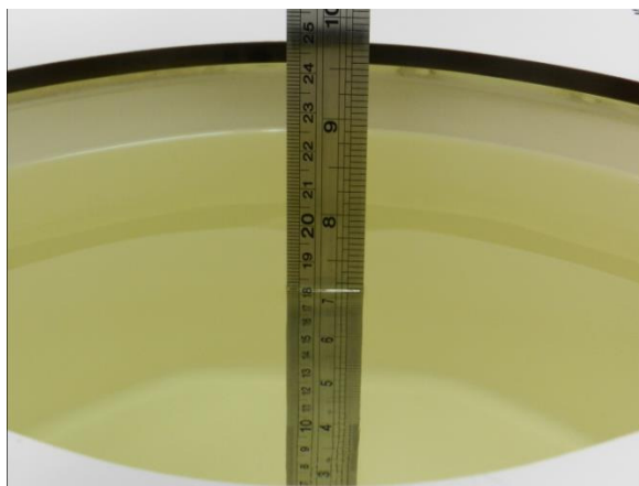
Fig 10.1 Photo of Liquid Height for Body SAR
