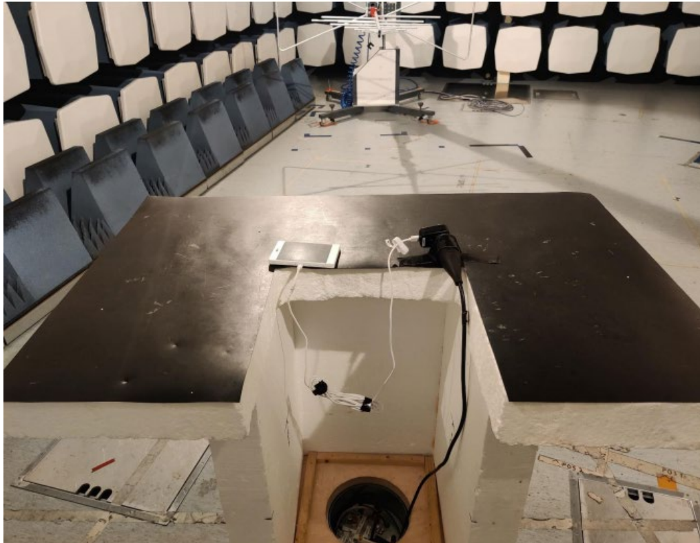
Radiated emission EUT setup back view, 30-1000MHz
