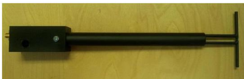
Figure 1 – MVG COMOSAR Validation Dipole
