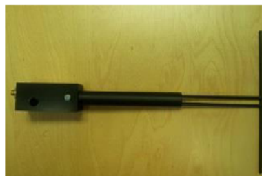
Figure 1 – MVG COMOSAR Validation Dipole
