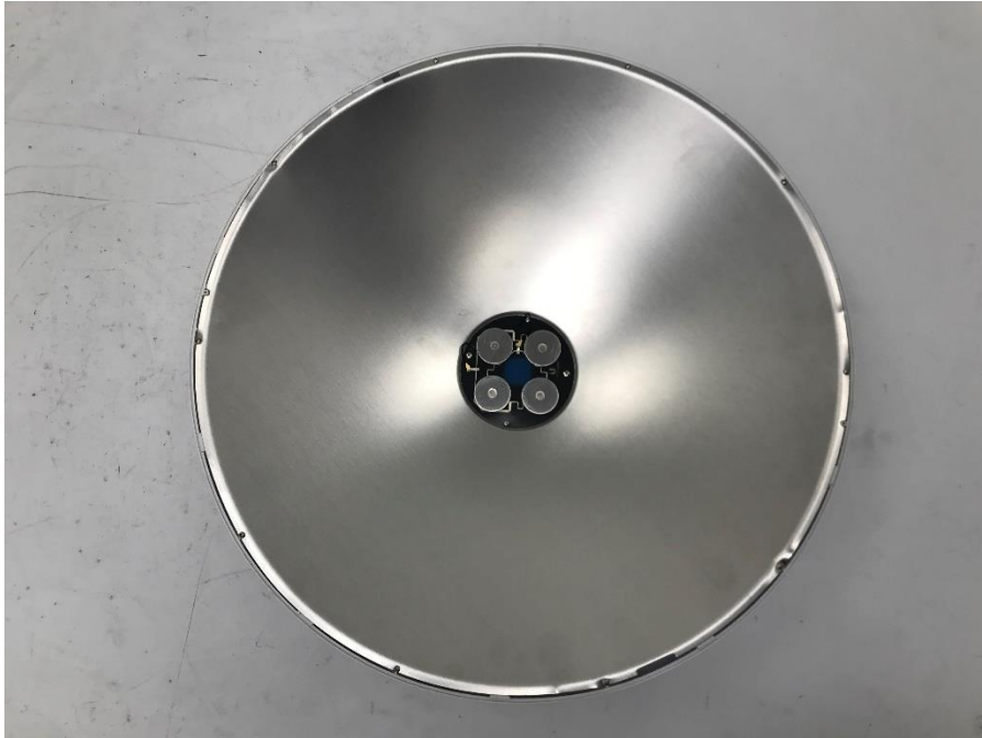
Photograph 1: Front View of DUT With Front Cover Off Showing Reflector
