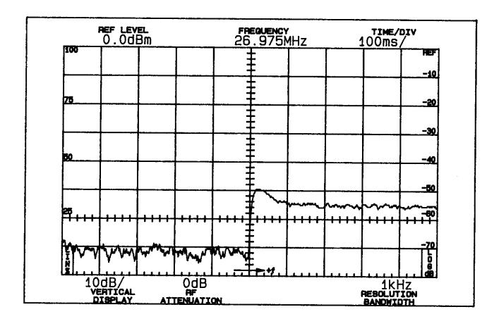
Measurement Conditions: 16 dB over 50% modulation level at 1150
