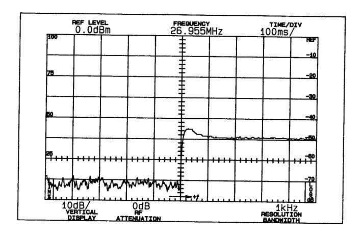
Measurement Conditions: 16 dB over 50% modulation level at 1150
