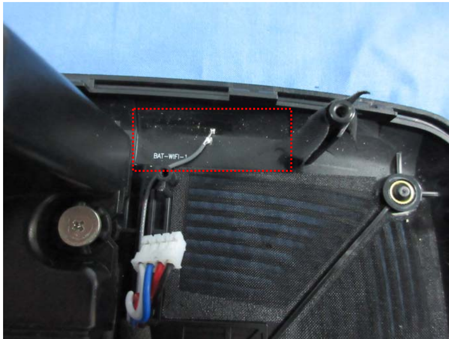
WiFi Antenna 1 View
