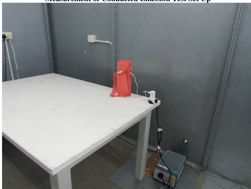
Measurement of Conducted Emission Test Set Up
