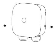
**Tighten** two M5 anti-theft screws to complete the installation.
