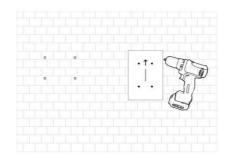
**Drill 8 Screw Holes** with a diameter of 0.35" and a depth of 2.05" by using 2 mounting templates. Please drill screw holes in the direction of the template arrow. And use two templates at a horizontal distance around 12 feet.
