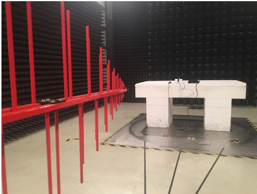
Radiated Emissions-Adapter power supply (Above 1GHz)
