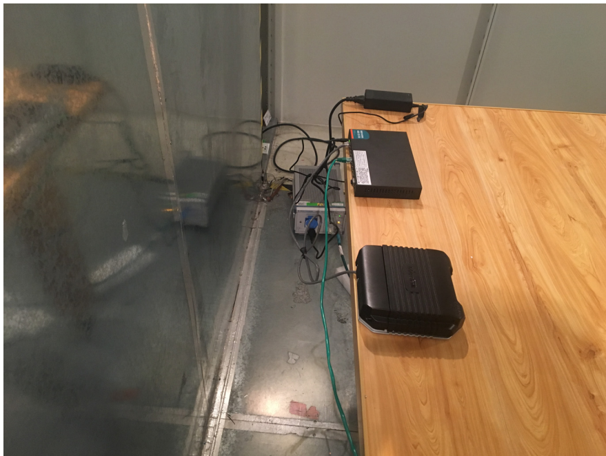
Conducted Emissions-POE power supply (Side View)
