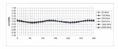
Axial Isotropy Error < ± 0.2 dB
