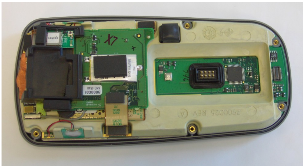
7900 “BUPE” Radio Placement Internal
