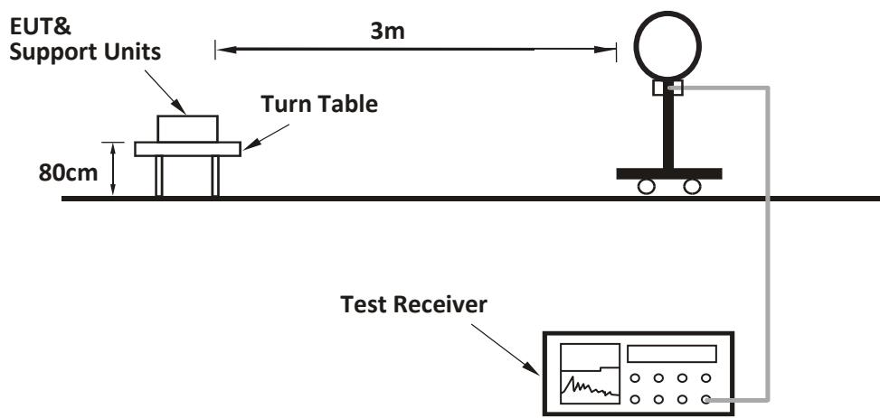
For Radiated emission 30MHz to 1GHz:
