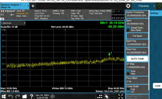
n77(3700~3980 MHz)\_40 M\_Conducted Spurious(Above10 G)\_Low\_BPSK\_1RB
