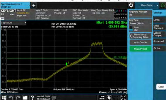
n77(3700~3980 MHz)\_20 M\_Band Edge\_Low\_BPSK\_1RB(1)
