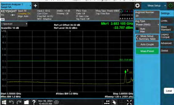
n77(3700~3980 MHz)\_20 M\_Band Edge\_Low\_BPSK\_1RB(3)
