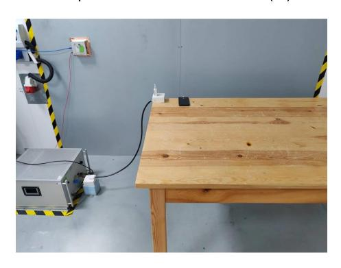
Set-up for Radiated Emission (RE), Below 1GHz
