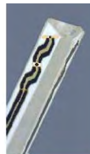
Figure G.2.2 Probe Thick-Film Technique
