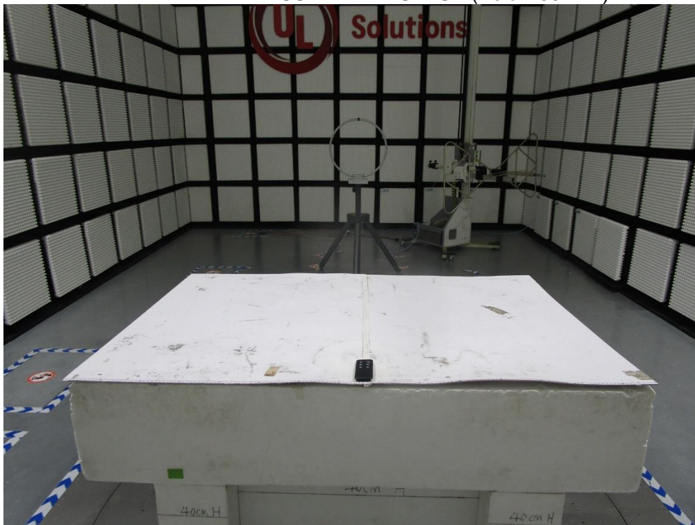
RADIATED RF MEASUREMENT SETUP (Below 30MHz)
