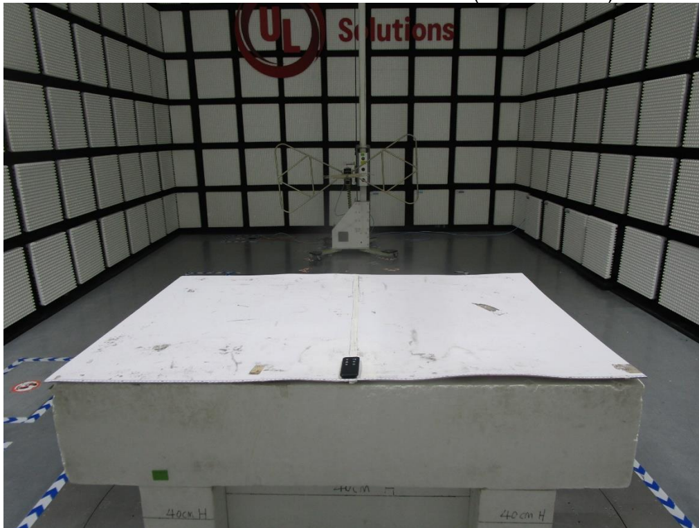
RADIATED RF MEASUREMENT SETUP (30MHz~1GHz)
