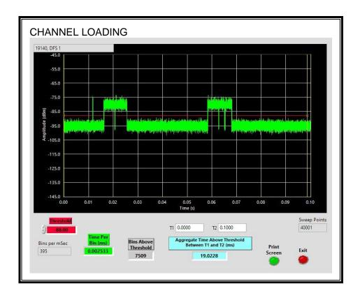
The level of traffic loading on the channel by the EUT is 19.023%
