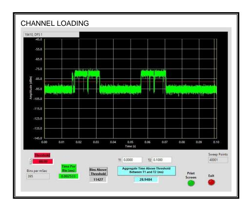
The level of traffic loading on the channel by the EUT is 28.95%
