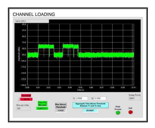
The level of traffic loading on the channel by the EUT is 28.97%
