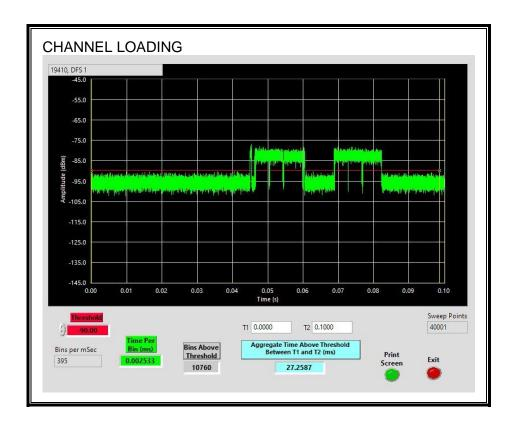
The level of traffic loading on the channel by the EUT is 27.25%
