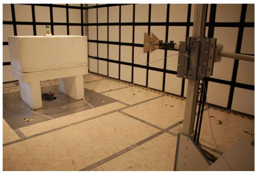
1.3. Radiated Emission test setup photo for BT/BT LE/WLAN 2.4GHz (ANSI C63.10: 2013)
