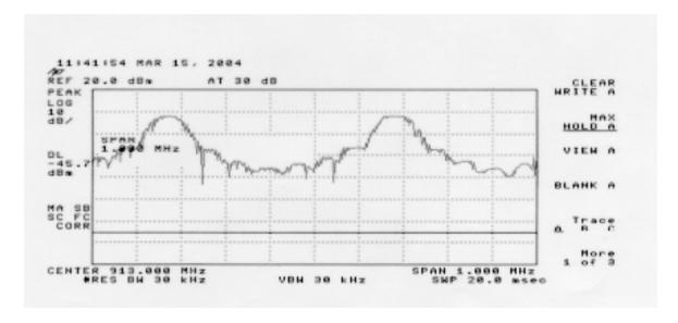
Spectrum Plot 1 shows two adjacent channels with modulation. Compliance with section 15.247(a)(1) is demonstrated with a test sample configured with firmware allowing two adjacent channels to be captured. Plot 1 also shows the 20 dB bandwidth of a single channel of 300 kHz, to demonstrate compliance with 15.247(a)(1)(i).
