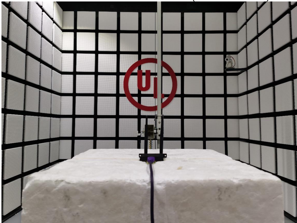
RADIATED RF MEASUREMENT SETUP (Above 1G – X axis)
