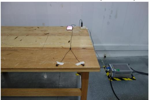
1.2 Radiated Emissions (9KHz-30MHz) Test Setup
