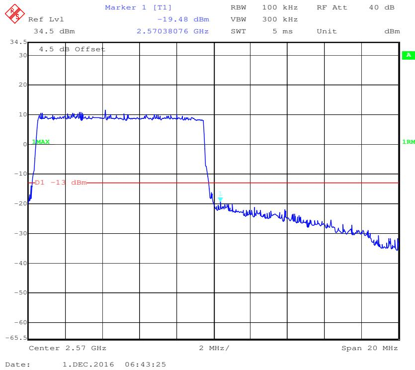
**16-QAM (10.0 MHz, FULL RB) - Left Band Edge**
