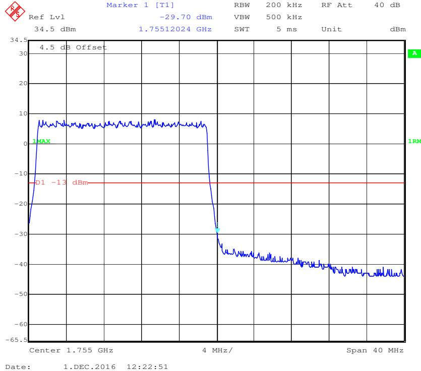
**LTE Band 5:****QPSK (1.4 MHz, FULL RB) - Left Band Edge**
