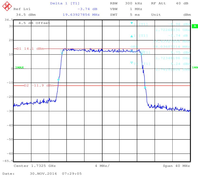
**16-QAM (20.0 MHz) - 99% Occupied & 26 dB Emissions Bandwidth, Middle channel**
