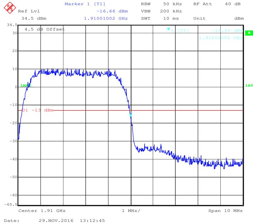
**PCS Band, Left Band Edge for HSDPA (16QAM) Mode**
