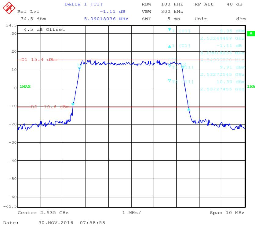
**16-QAM (5.0 MHz) - 99% Occupied & 26 dB Emissions Bandwidth, Middle channel**
