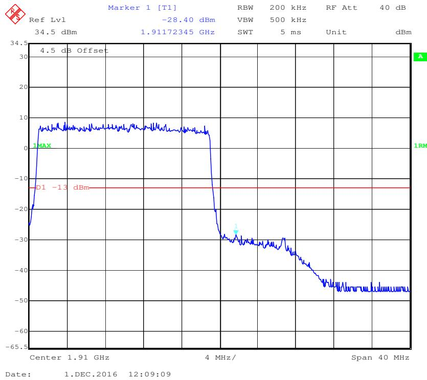
**LTE Band 4:****QPSK (1.4 MHz, FULL RB) - Left Band Edge**
