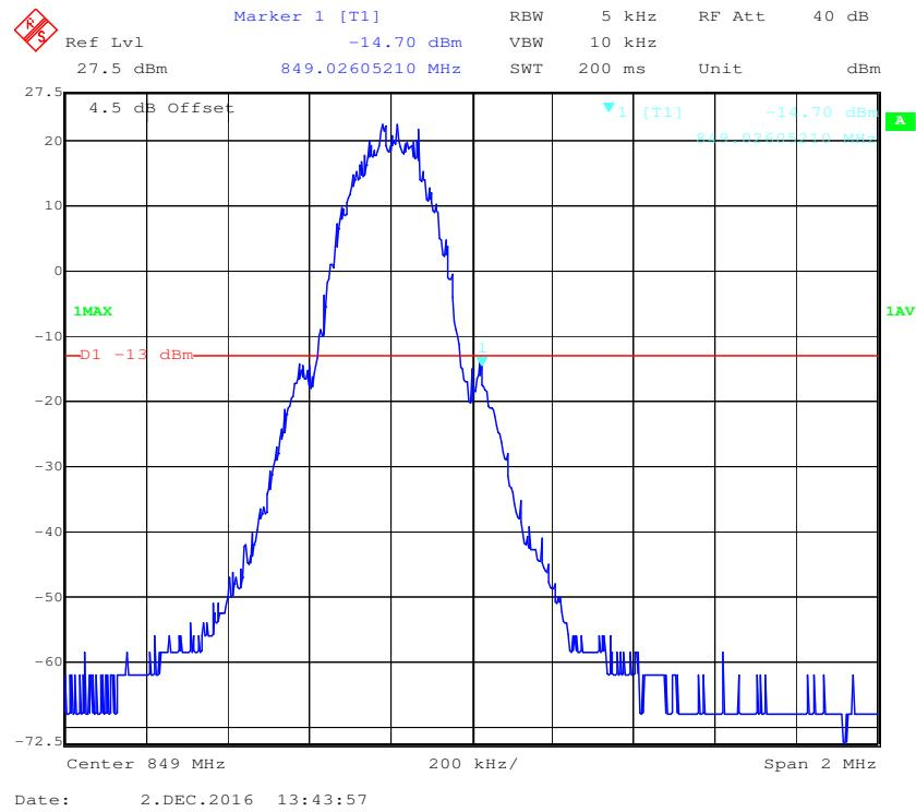
**Cellular Band, Left Band Edge for EDGE Mode**
