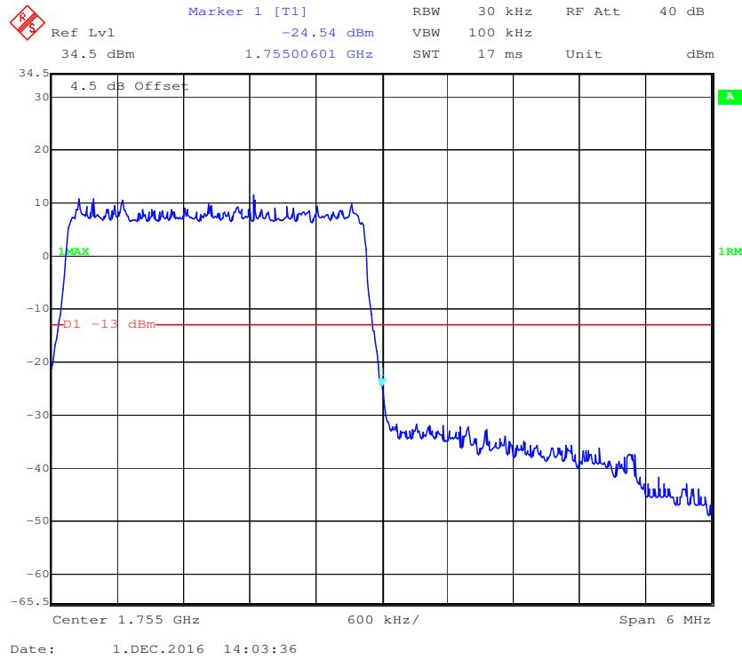
**16-QAM (3.0 MHz, FULL RB) - Left Band Edge**
