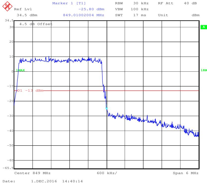
**QPSK (5.0 MHz, FULL RB) - Left Band Edge**
