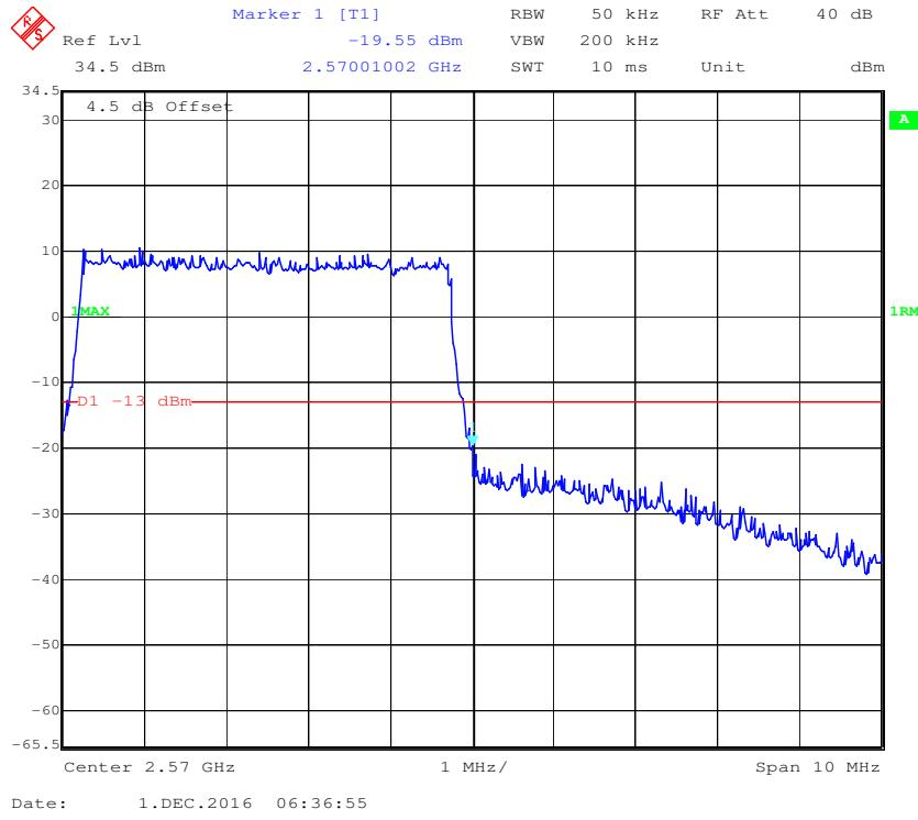
**QPSK (10.0 MHz, FULL RB) - Left Band Edge**
