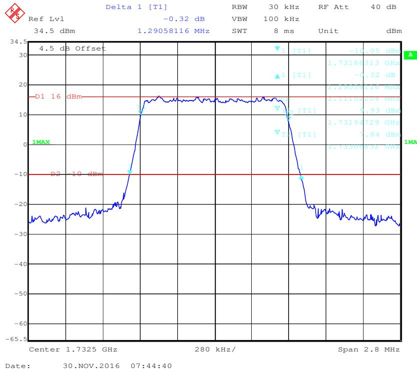
**16-QAM (1.4 MHz) - 99% Occupied Bandwidth &26 dB Bandwidth, Middle channel**
