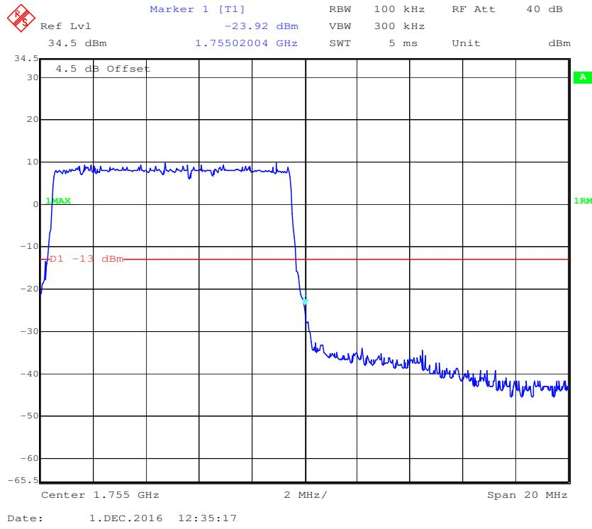
**16-QAM (10.0 MHz, FULL RB) - Left Band Edge**
