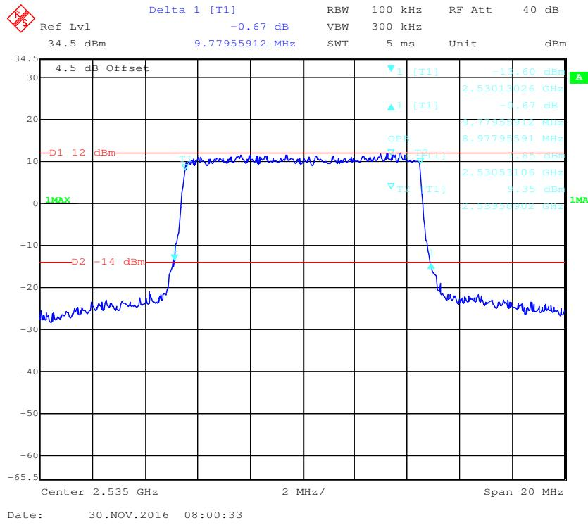
**16-QAM (10.0 MHz) - 99% Occupied & 26 dB Emissions Bandwidth, Middle channel**
