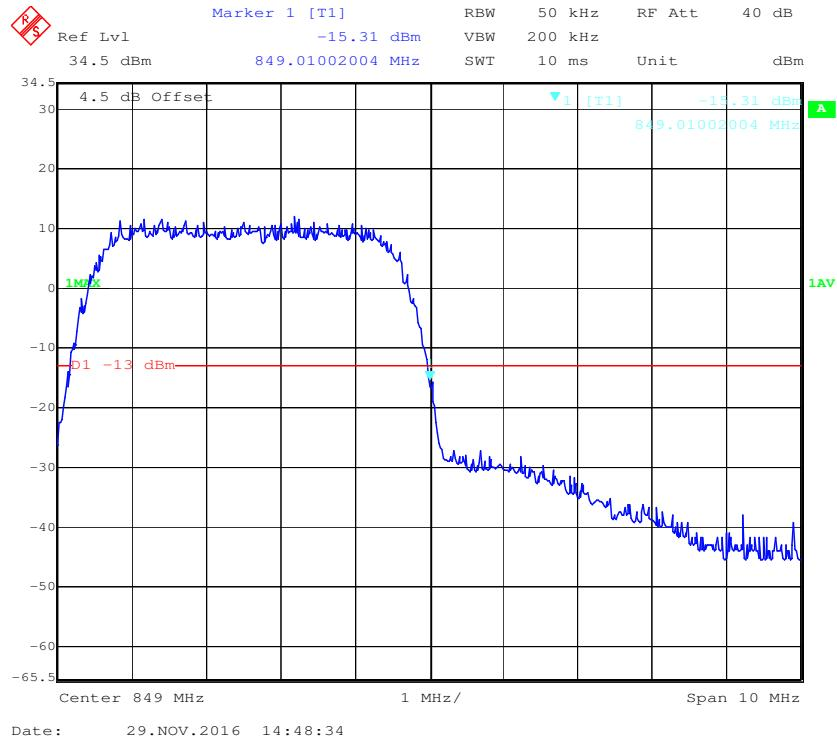
**Cellular Band, Left Band Edge for HSUPA (BPSK) Mode**
