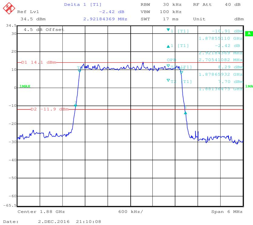
**16-QAM (3.0 MHz) - 99% Occupied Bandwidth &26 dB Bandwidth, Middle channel**
