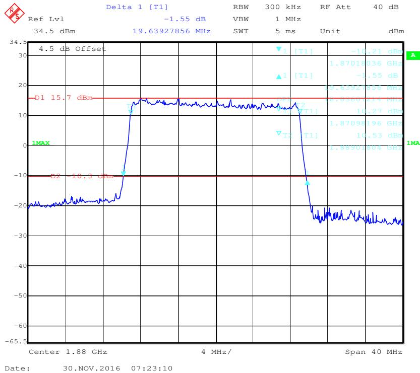
**16-QAM (20.0 MHz) - 99% Occupied & 26 dB Emissions Bandwidth, Middle channel**
