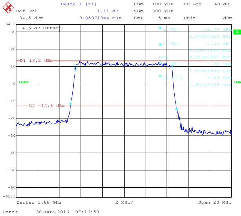
**16-QAM (10.0 MHz) - 99% Occupied & 26 dB Emissions Bandwidth, Middle channel**
