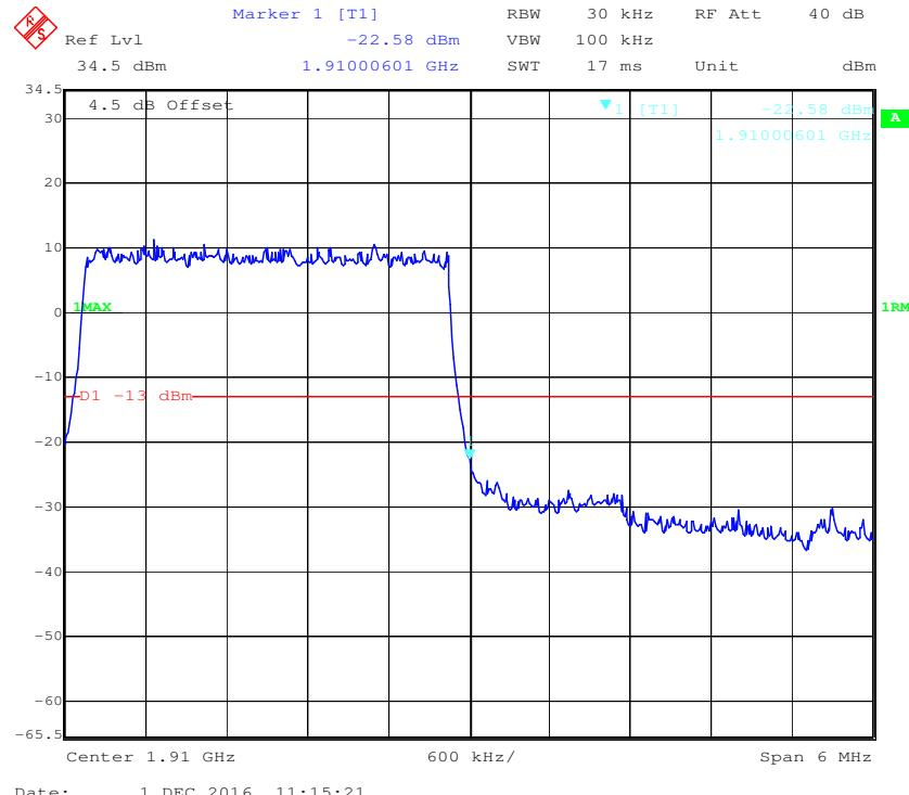
**16-QAM (3.0 MHz, FULL RB) - Left Band Edge**
