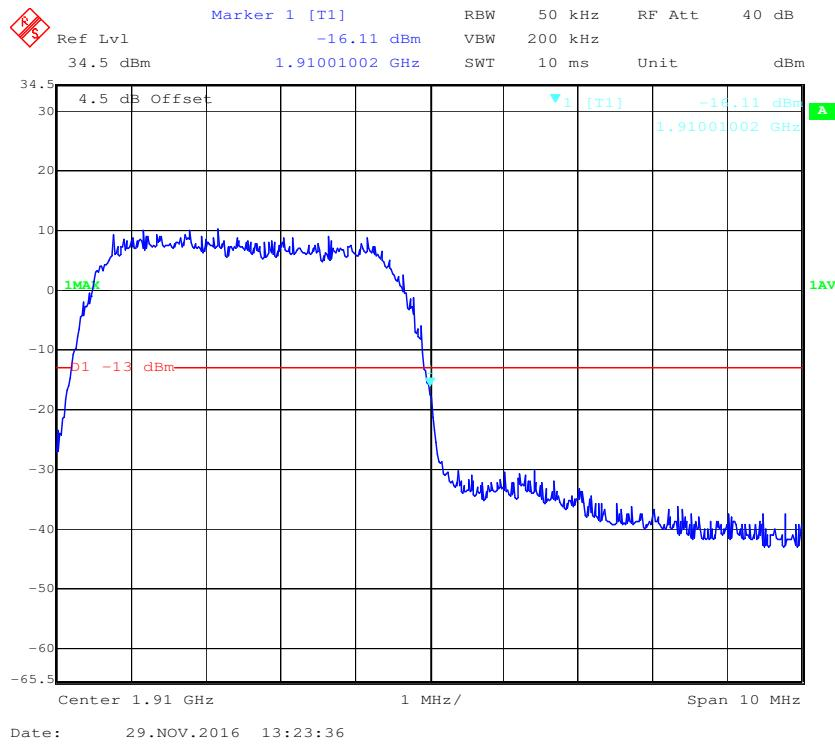
**LTE Band 2:****QPSK (1.4 MHz, FULL RB) - Left Band Edge**
