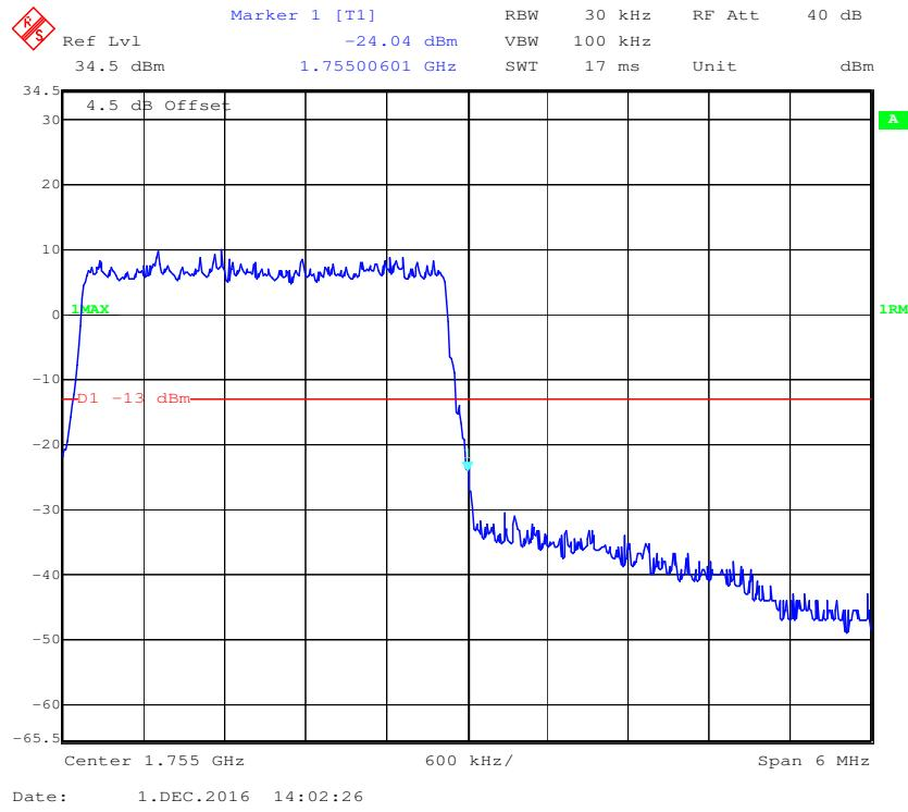
**QPSK (5.0 MHz, FULL RB) - Left Band Edge**
