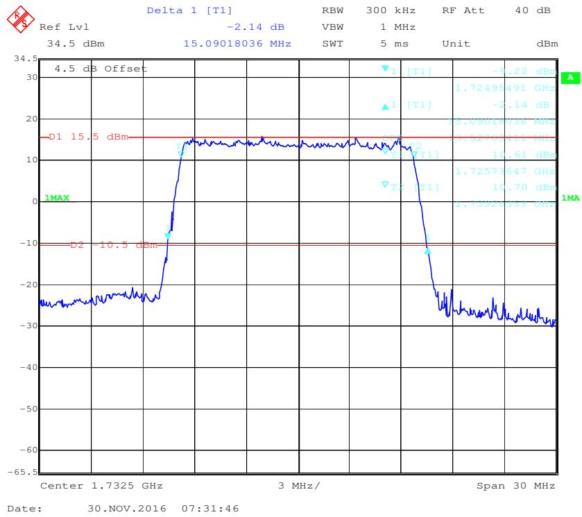
**16-QAM (15.0 MHz) - 99% Occupied & 26 dB Emissions Bandwidth, Middle channel**
