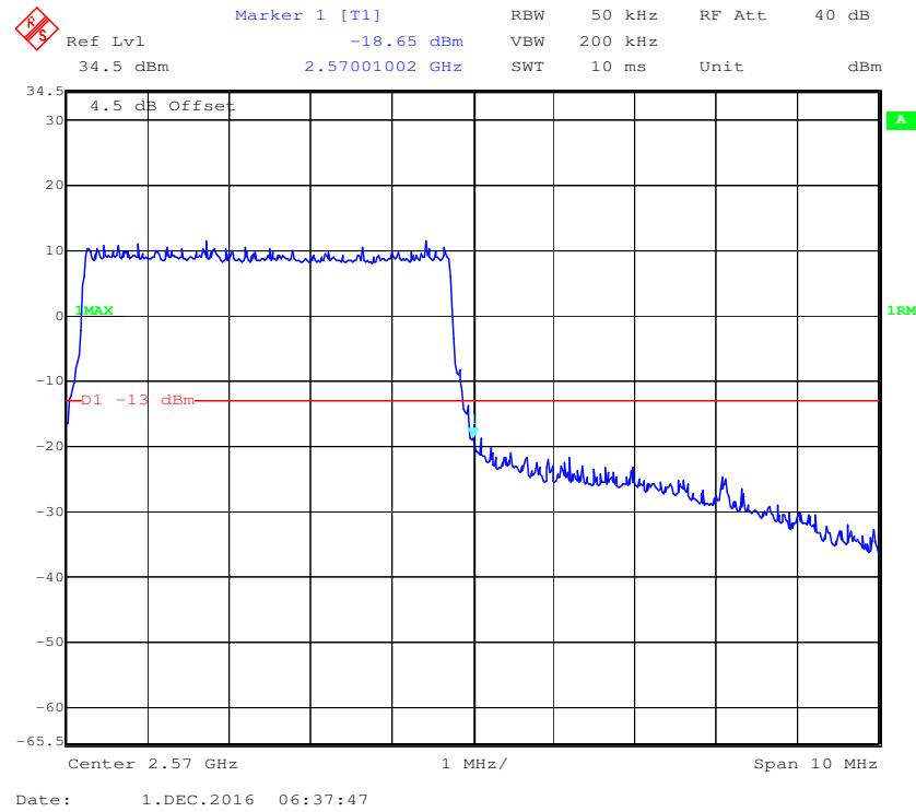
**16-QAM (5.0 MHz, FULL RB) - Left Band Edge**
