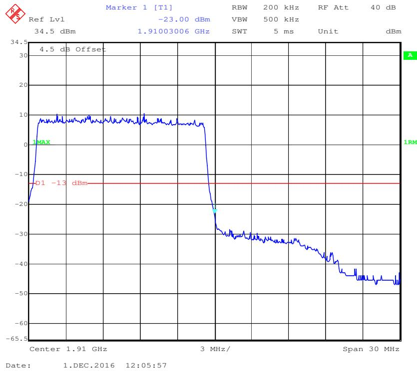
**QPSK (20.0 MHz, FULL RB) - Left Band Edge**
