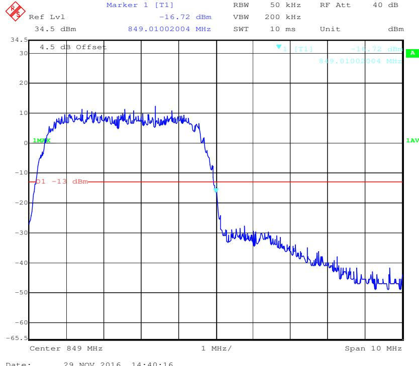
**PCS Band, Left Band Edge for GSM (GMSK) Mode**
