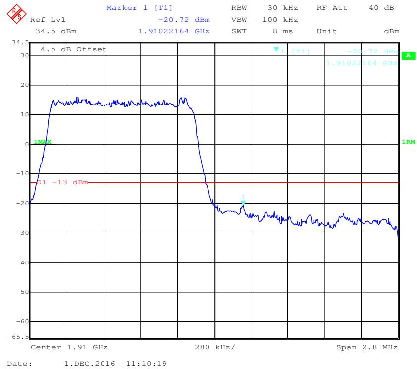
**16-QAM (1.4 MHz, FULL RB) - Left Band Edge**
