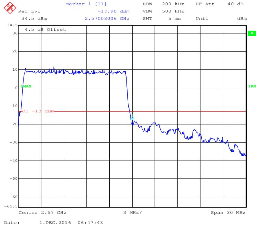
**16-QAM (15 MHz, FULL RB) - Left Band Edge**
