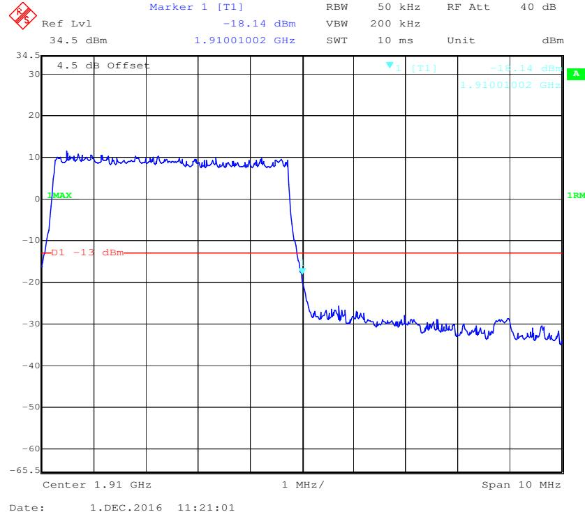
**QPSK (10.0 MHz, FULL RB) - Left Band Edge**
