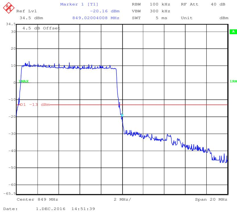
**16-QAM (10.0 MHz, FULL RB) - Left Band Edge**
