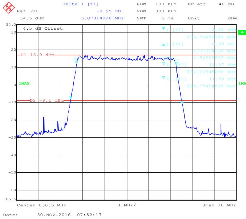
**16-QAM (5.0 MHz) - 99% Occupied & 26 dB Emissions Bandwidth, Middle channel**
