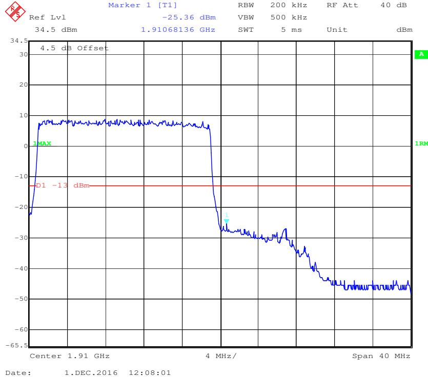
**16-QAM (20.0 MHz, FULL RB) - Left Band Edge**
