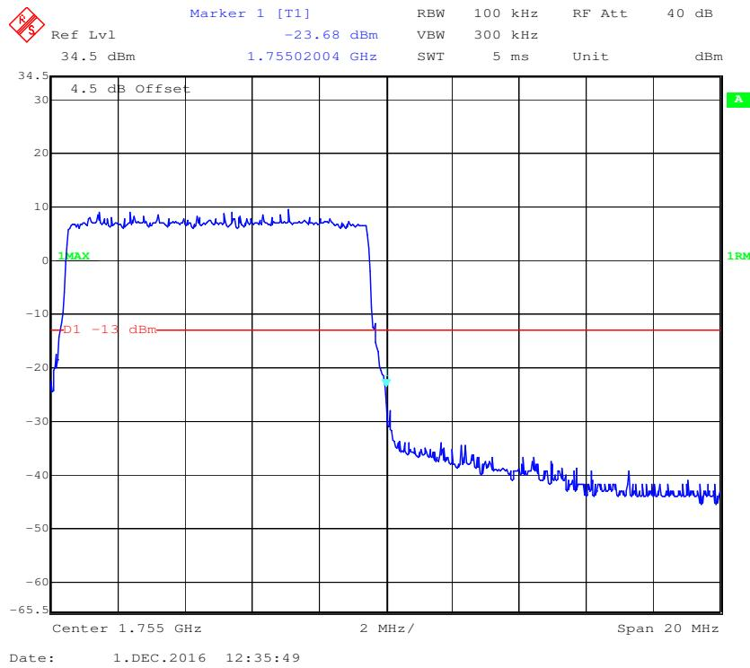
**QPSK (15.0 MHz, FULL RB) - Left Band Edge**
