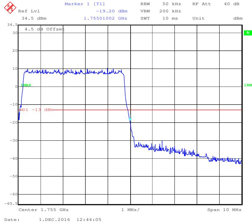
**16-QAM (5.0 MHz, FULL RB) - Left Band Edge**
