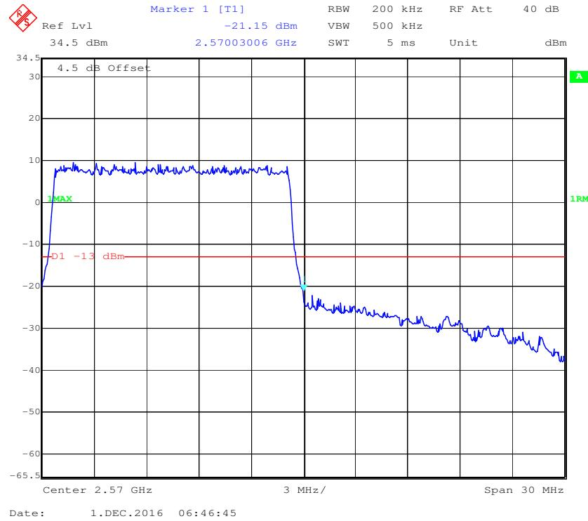
**QPSK (20 MHz, FULL RB) - Left Band Edge**
