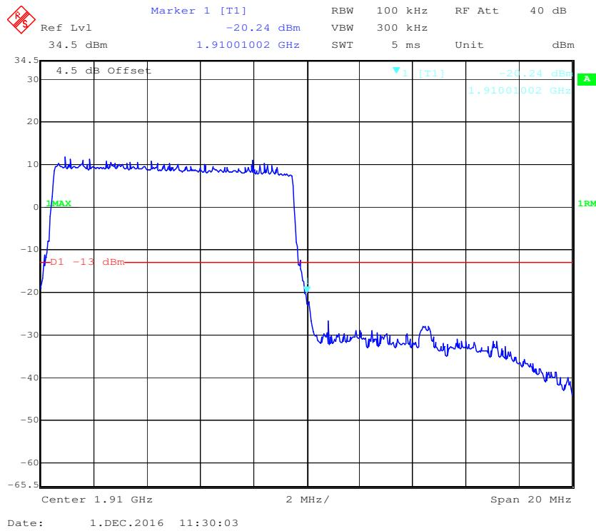
**16-QAM (10.0 MHz, FULL RB) - Left Band Edge**
