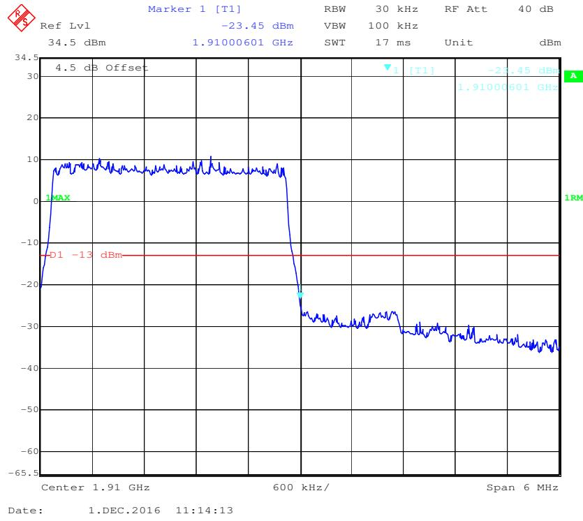
**QPSK (5.0 MHz, FULL RB) - Left Band Edge**
