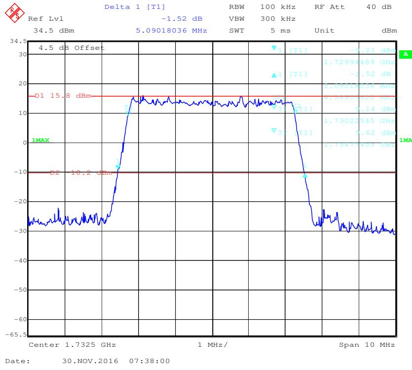
**16-QAM (5.0 MHz) - 99% Occupied & 26 dB Emissions Bandwidth, Middle channel**
