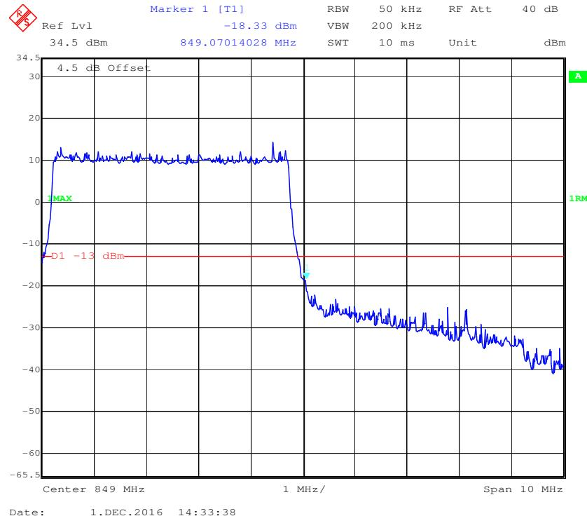
**16-QAM (5.0 MHz, FULL RB) - Left Band Edge**
