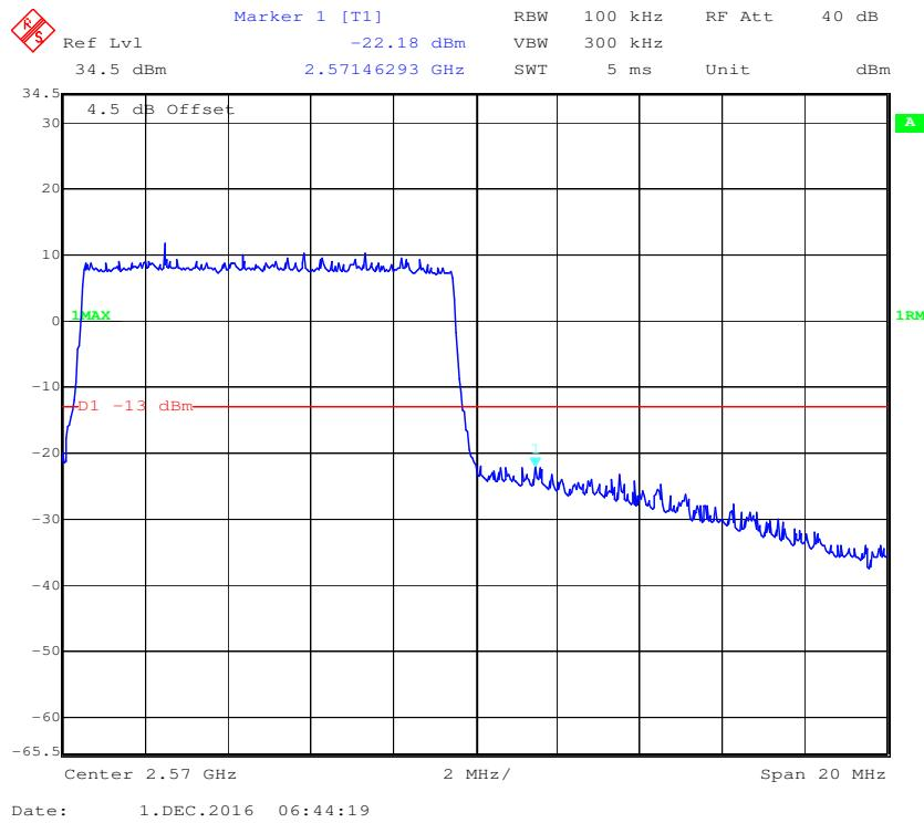
**QPSK (15 MHz, FULL RB) - Left Band Edge**
