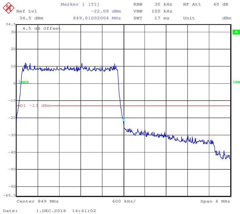
**16-QAM (3.0 MHz, FULL RB) - Left Band Edge**
