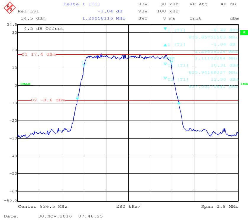
**16-QAM (1.4 MHz) - 99% Occupied Bandwidth &26 dB Bandwidth, Middle channel**
