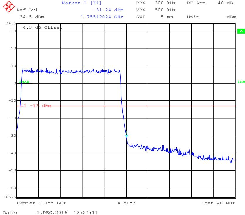
**16-QAM (20.0 MHz, FULL RB) - Left Band Edge**
