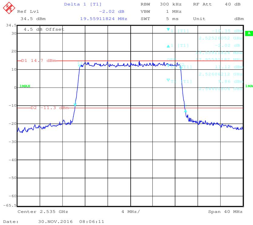
**16-QAM (20.0 MHz) - 99% Occupied & 26 dB Emissions Bandwidth, Middle channel**
