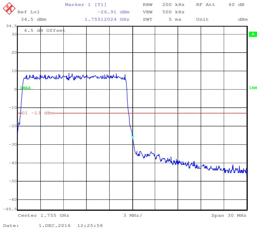
**QPSK (20.0 MHz, FULL RB) - Left Band Edge**
