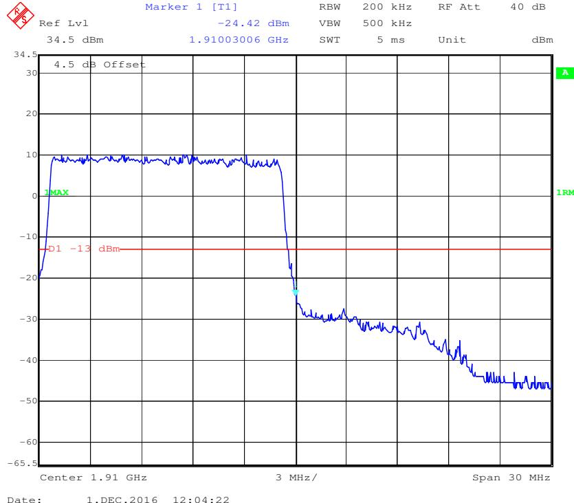
**16-QAM (15.0 MHz, FULL RB) - Left Band Edge**
