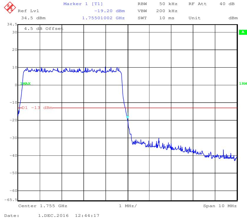
**QPSK (10.0 MHz, FULL RB) - Left Band Edge**
