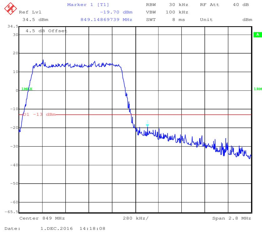
**QPSK (3.0 MHz, FULL RB) - Left Band Edge**
