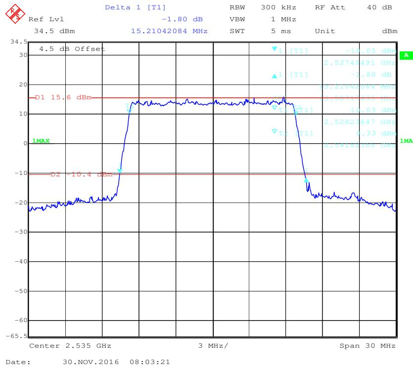
**16-QAM (15.0 MHz) - 99% Occupied & 26 dB Emissions Bandwidth, Middle channel**
