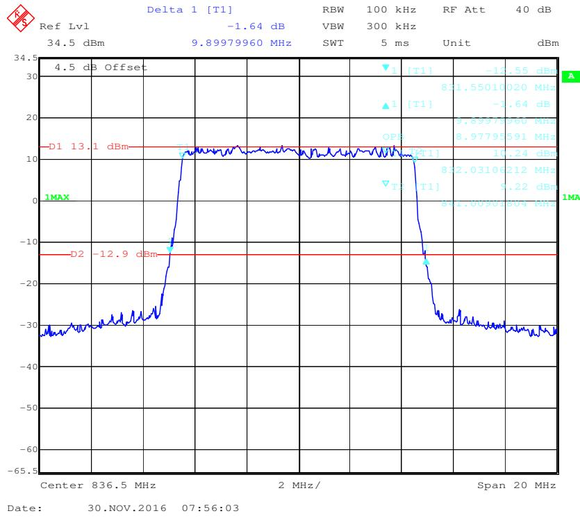
**16-QAM (10.0 MHz) - 99% Occupied & 26 dB Emissions Bandwidth, Middle channel**
