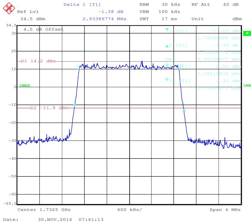
**16-QAM (3.0 MHz) - 99% Occupied Bandwidth &26 dB Bandwidth, Middle channel**
