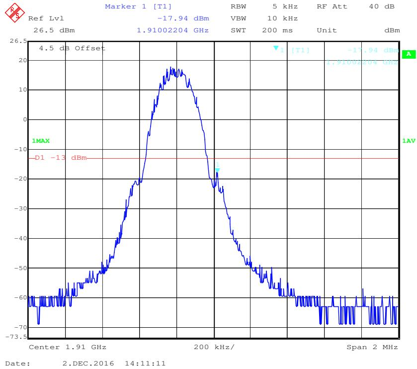
**PCS Band, Left Band Edge for EDGE Mode**
