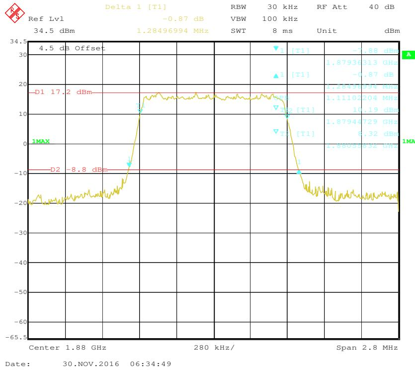
**16-QAM (1.4 MHz) - 99% Occupied Bandwidth &26 dB Bandwidth, Middle channel**
