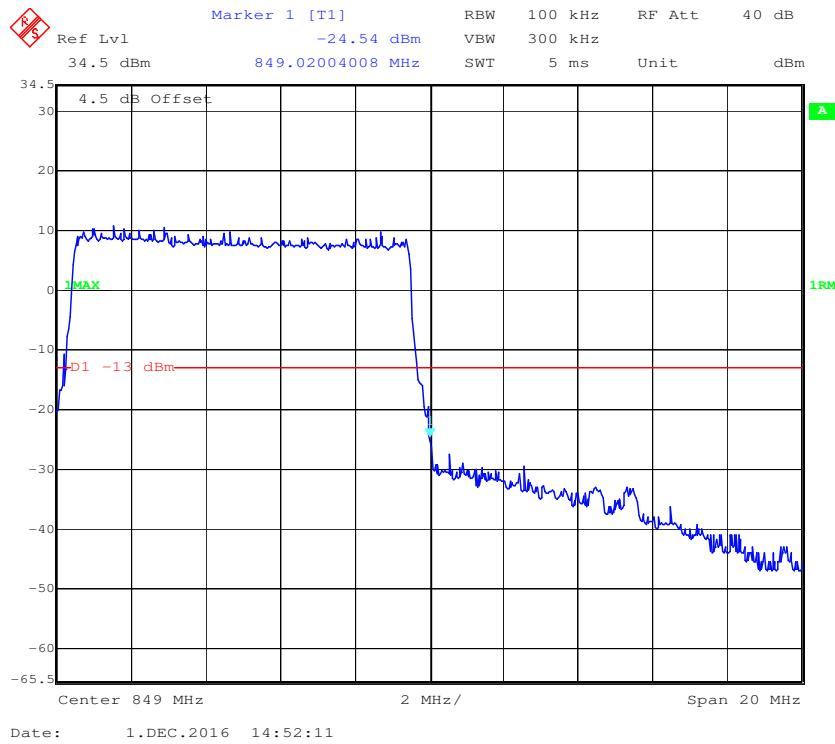
**LTE Band 7:****QPSK (5.0 MHz, FULL RB) - Left Band Edge**
