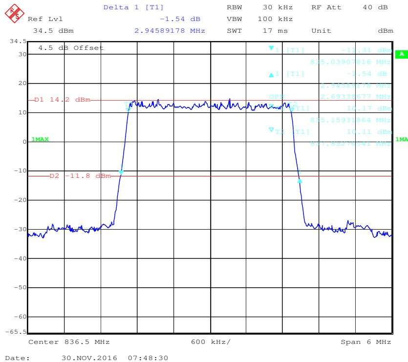
**16-QAM (3.0 MHz) - 99% Occupied Bandwidth &26 dB Bandwidth, Middle channel**
