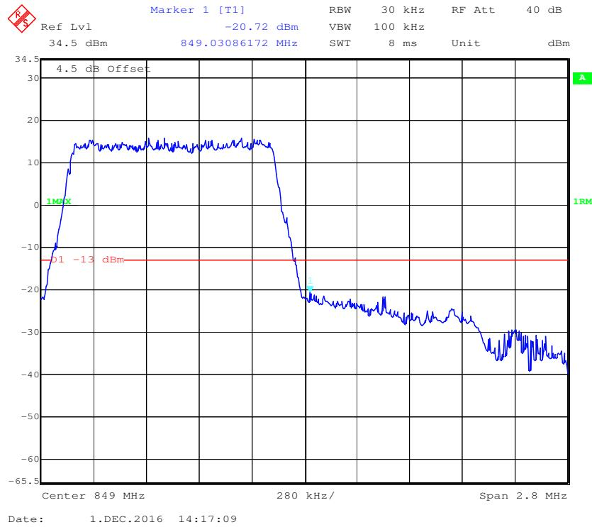
**16-QAM (1.4 MHz, FULL RB) - Left Band Edge**
