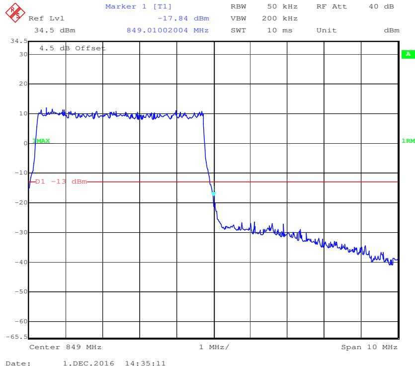
**QPSK (10.0 MHz, FULL RB) - Left Band Edge**
