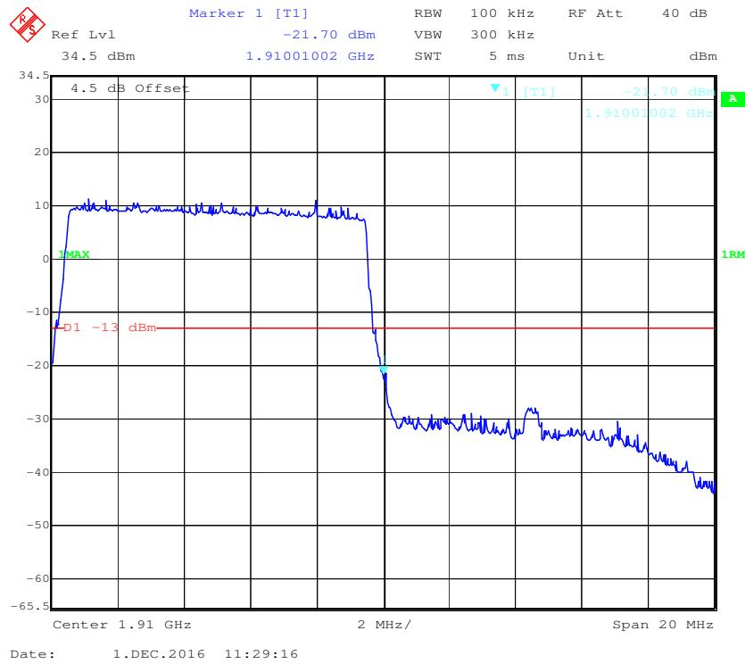
**QPSK (15.0 MHz, FULL RB) - Left Band Edge**
