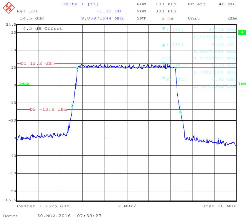
**16-QAM (10.0 MHz) - 99% Occupied & 26 dB Emissions Bandwidth, Middle channel**
