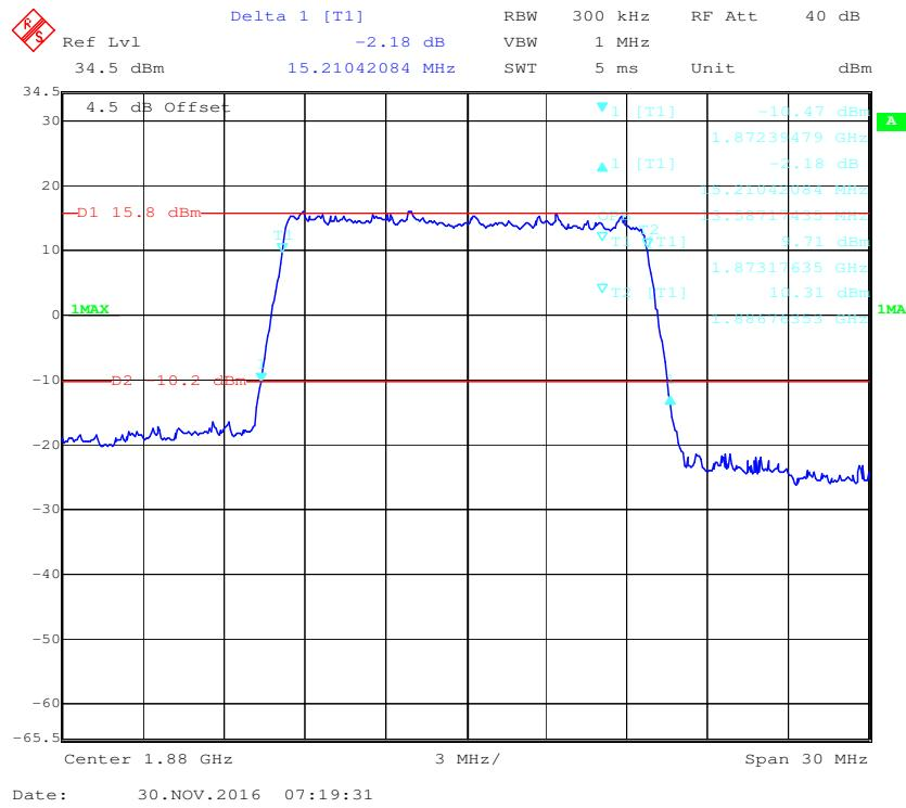
**16-QAM (15.0 MHz) - 99% Occupied & 26 dB Emissions Bandwidth, Middle channel**
