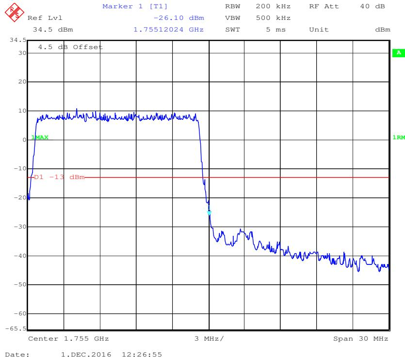
**16-QAM (15.0 MHz, FULL RB) - Left Band Edge**
