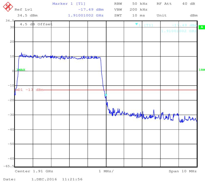
**16-QAM (5.0 MHz, FULL RB) - Left Band Edge**
