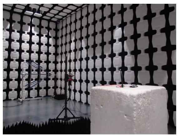
Description: Substitution Antenna for EIRP Test
