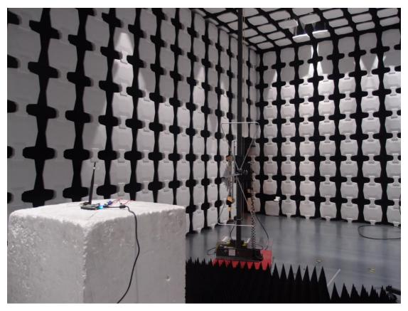
Description: Substitution Antenna for ERP Test
