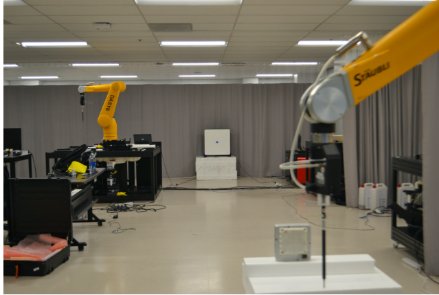
Figure 3 - Test setup example: 10m separation distance
