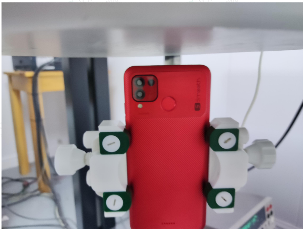
10mm body-worn Top Side Setup Photo (hotspot)
