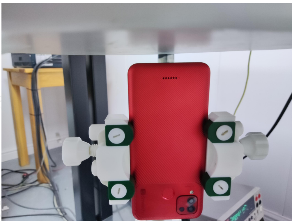
10mm body-worn Bottom Side Setup Photo (hotspot)
