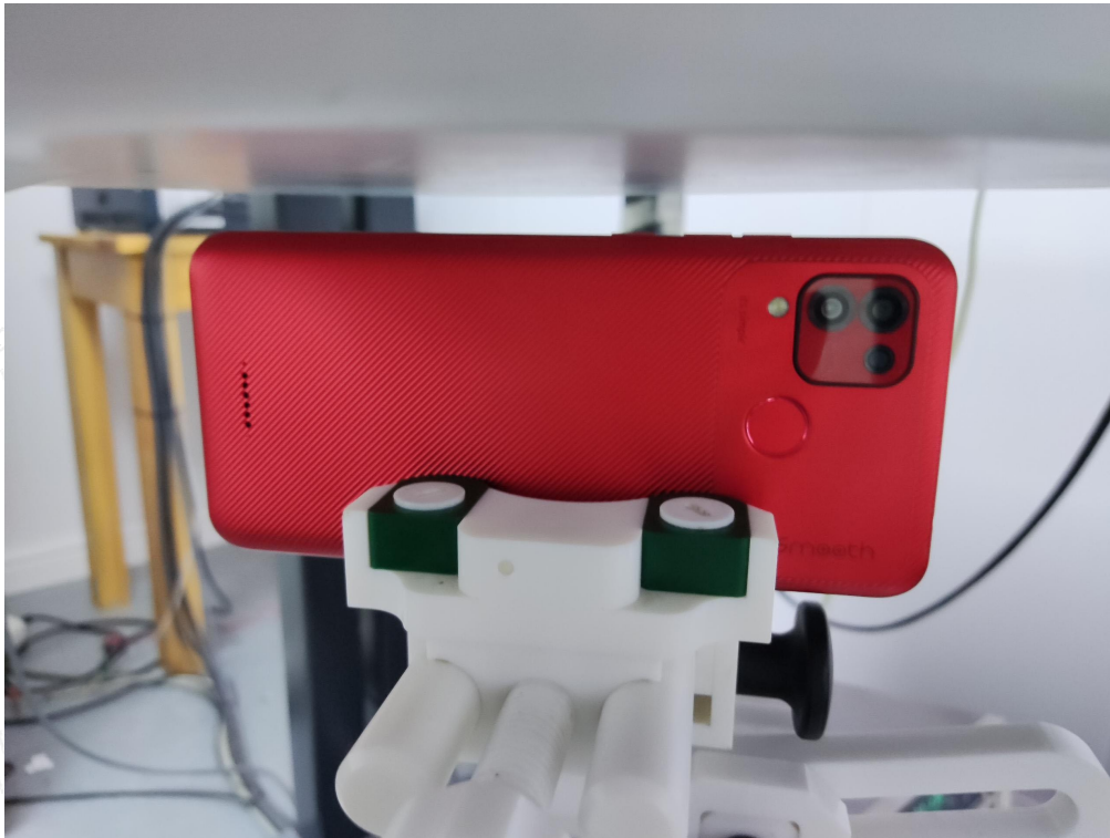
10mm body-worn Right Side Setup Photo (hotspot)
