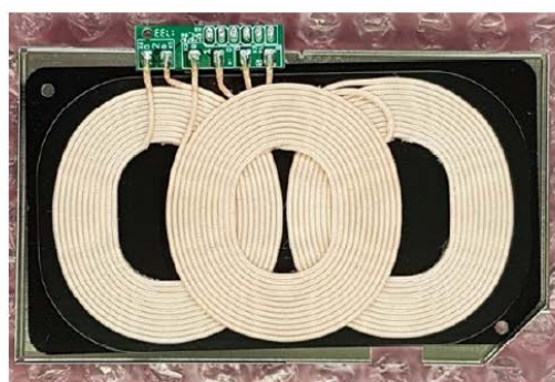
Charging coil element with connector, ferrite plate and metal shield, view from top and bottom side.
