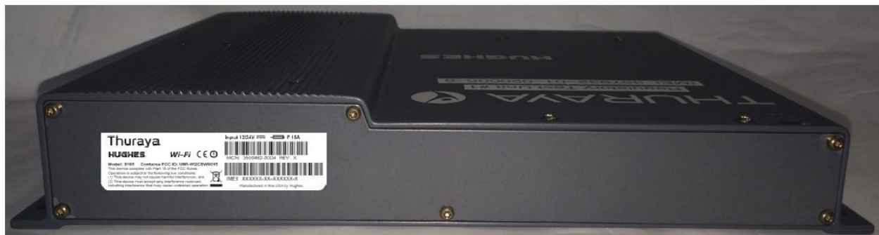
Fig 2. Thuraya 9105 BDU – Chassis label location
