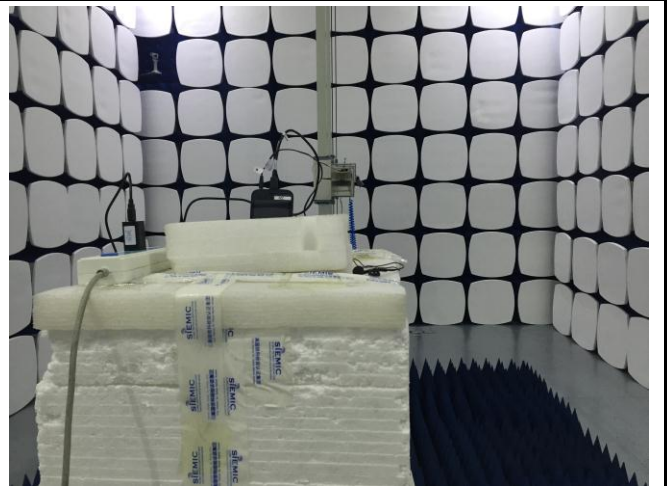
Radiated Spurious Emissions Test Setup Above 1GHz
