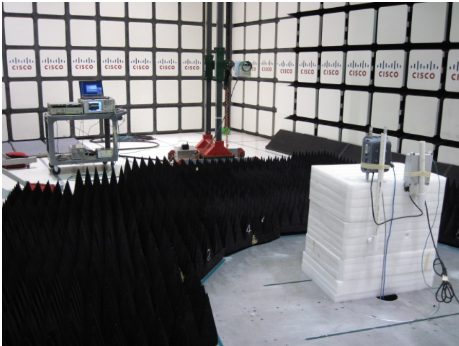
Radiated Test Setup 18–40GHz
