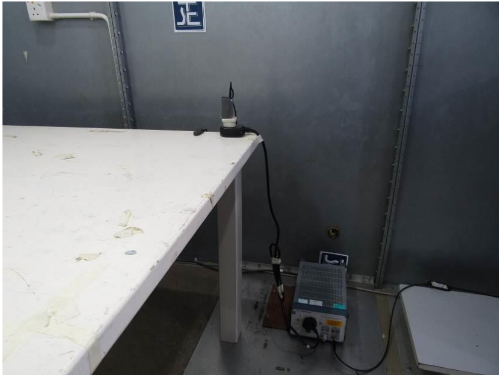
Measurement of Conducted Emission Test Set Up
