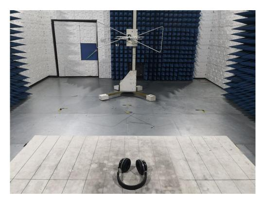
RADIATED EMISSION TEST SETUP ABOVE 1GHZ
