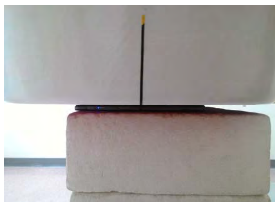
Fig.4 EUT Back side to flat phantom
