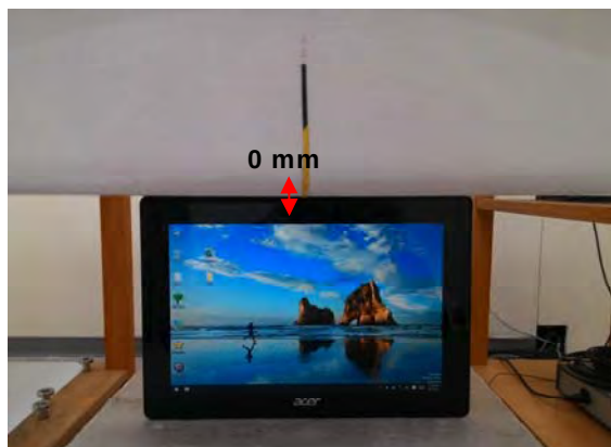
Fig.3 EUT Top side to flat phantom
