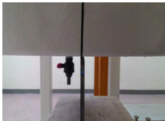
Fig.3 EUT Top side to flat phantom
