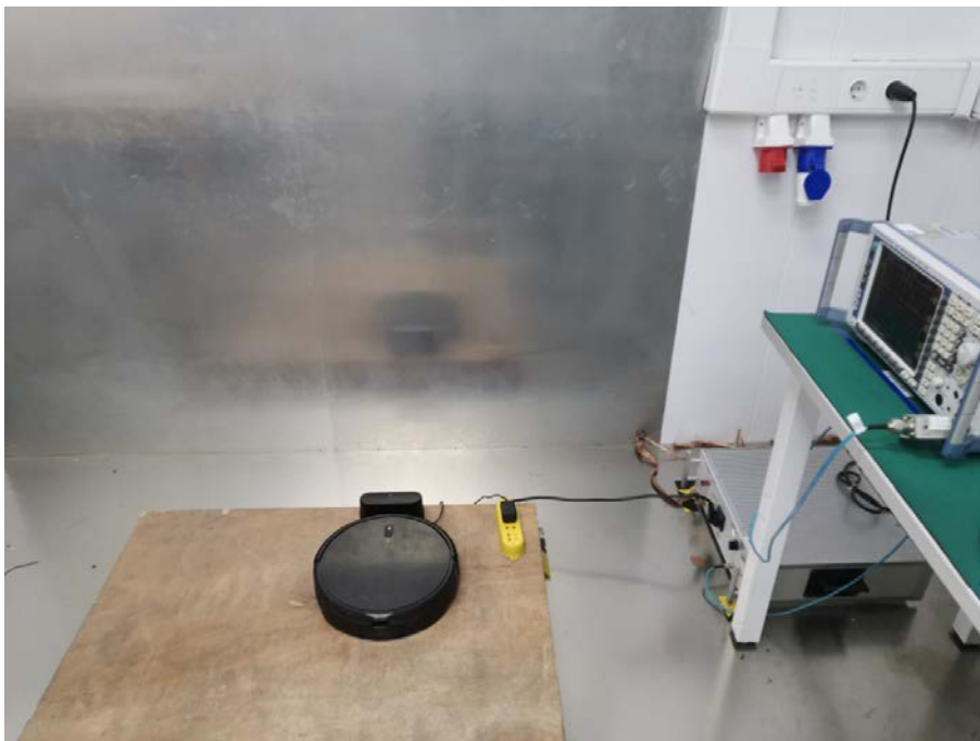
Adapter 1: Conducted emissions
