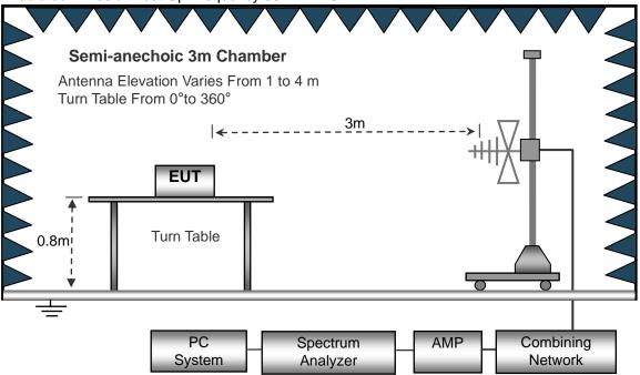
(C) Radiated Emission Test-Up Frequency Above 1GHz
