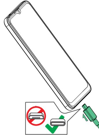
EN Insert Type-C cable to charge
