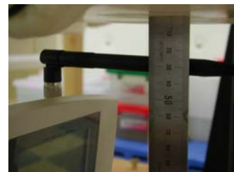
Fig. 21. Body SAR Test Setup with Holster
